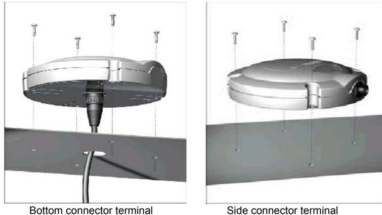
A mounting template is included to be used to perforate the installation surface. It is highly recommended to install the terminal with blocking nuts in order to avoid vibrations due to looseness of those nuts.
