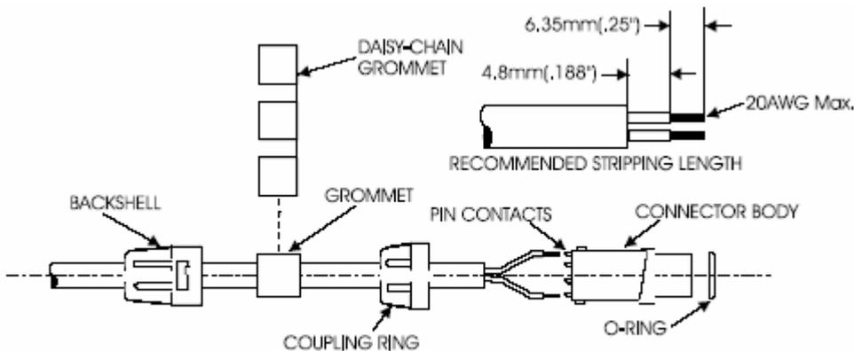
Figure 14: Coaxial Mini-con-x Series Cable connector Assembly
